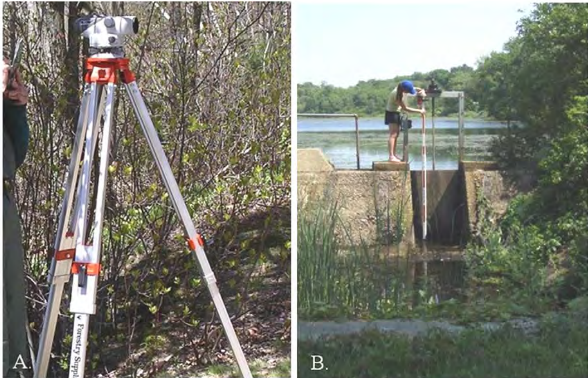
Figure 29. Examples of auto level and tripod used for elevation survey (A) and permanent structure used as a benchmark (B).
