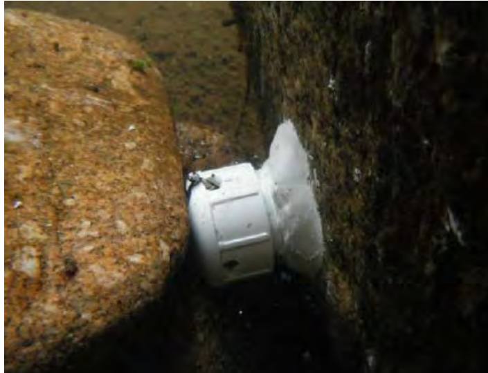
Figure 8. Close-up of a PVC solar shield with a temperature sensor glued to a rock in a stream. The rocks propped against the front of the solar shield holds it in place while the epoxy sets during the first 24 hours.
