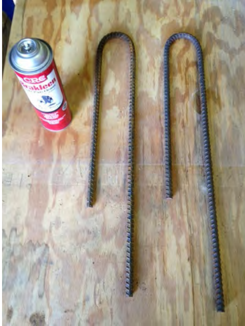
Figure 11. Using bent rebar for rebar installations has several advantages. It is more secure because the metal bar is anchored in two places. It also poses less safety risk for people who are wading through the stream because no sharp points protrude upward into the water column. This design was provided by Christopher M. Harbort, Principal Engineer, Waterborne Environmental, Inc. Champaign, IL. www.waterborne-env.com . Installations are easier if one leg is a little longer than the other because you can start the longer leg first and then pound the rest into place.
