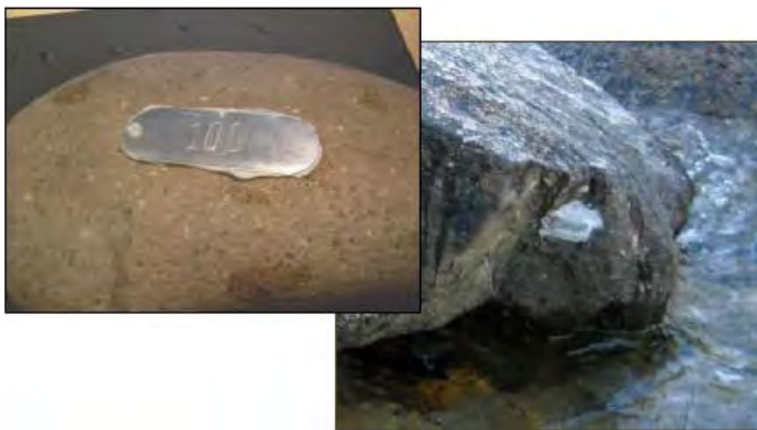
Figure 15. Metal forestry tags can be attached to the downstream side of large rocks to monument sites and air in relocation of sensors (Isaak et al. 2013).
