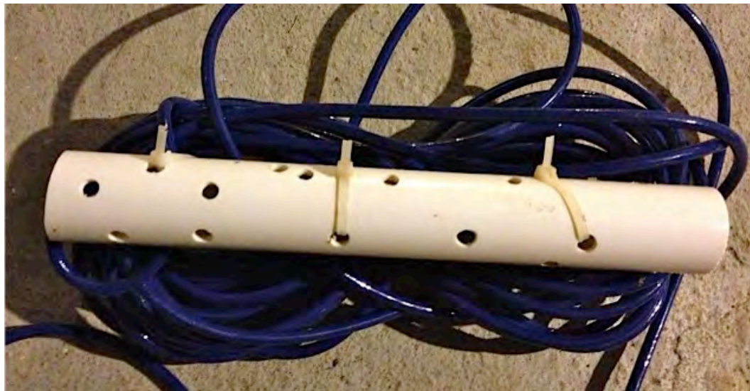
Figure 18. Example of a protective housing made of PVC pipe. This one is for a vented pressure transducer, which is secured inside the pipe with zip ties.
