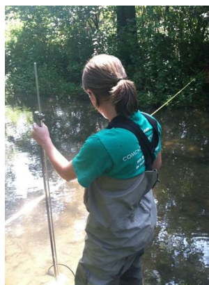
Fig. 22 (a) Manual discharge measurement being taken to develop a (b) rating curve at Slab Cabin Run - Upper (SLU)
