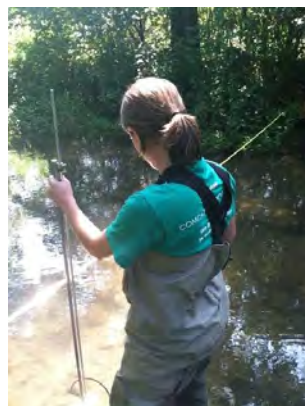
Fig. 31 (a) Manual discharge measurement being taken to develop a (b) rating curve at Slab Cabin Run - Upper (SLU)
