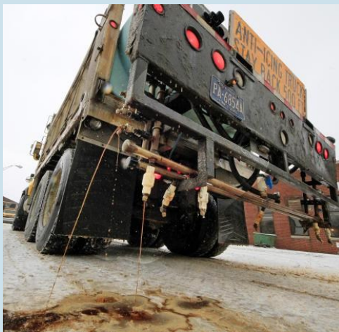
A PennDot deicing truck uses a mixture of brine and beet juice in 2014. Photo from: news.nationalgeographic.com
