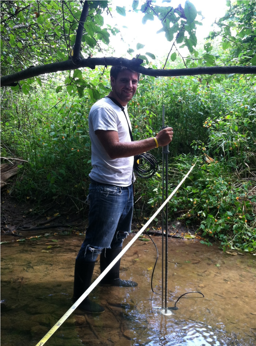
A WRMP volunteer takes discharge measurements at the Buffalo Run Upper site to help maintain the stage-discharge relationship for this monitoring location.
