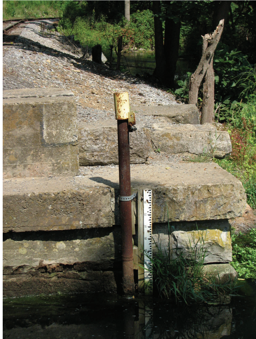
WRMP monitoring station on Logan Branch near Pleasant Gap (credit: B. Hutchison)
