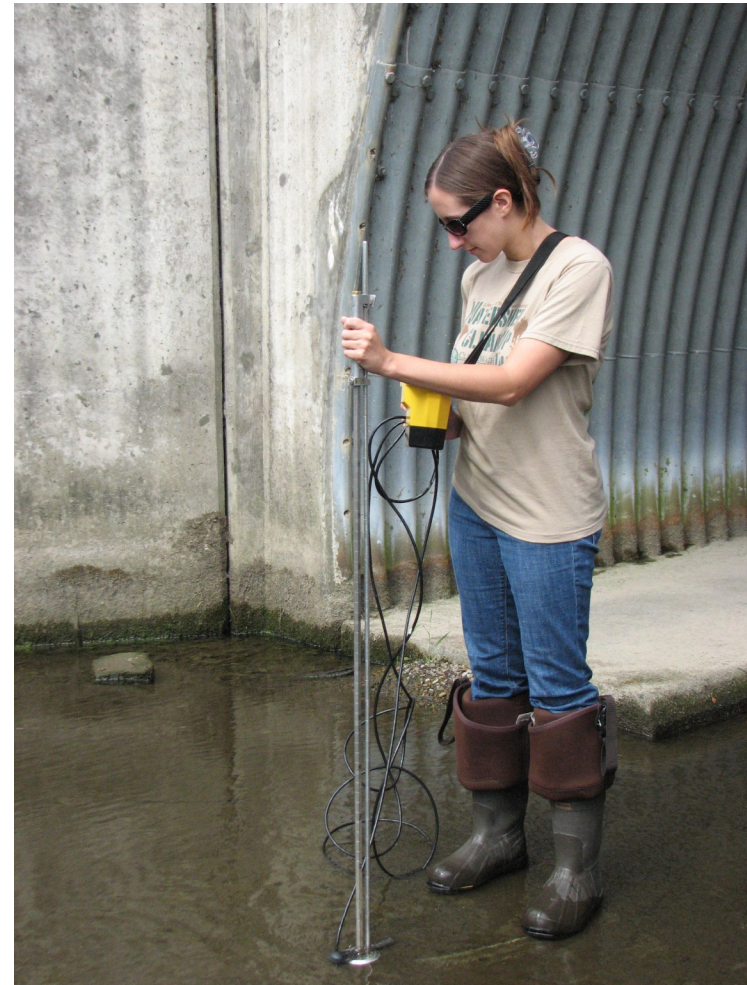
Water Resources Coordinator Brianna Hutchison takes an instantaneous flow measurement in Slab Cabin Run at E. College Avenue during summer low flow conditions (credit: S. Knorr)
