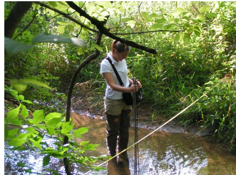
Water Resources Technician Nicole Rhodes takes a discharge measurement at the Buffalo Run Upper site (credit: G. Smith)
