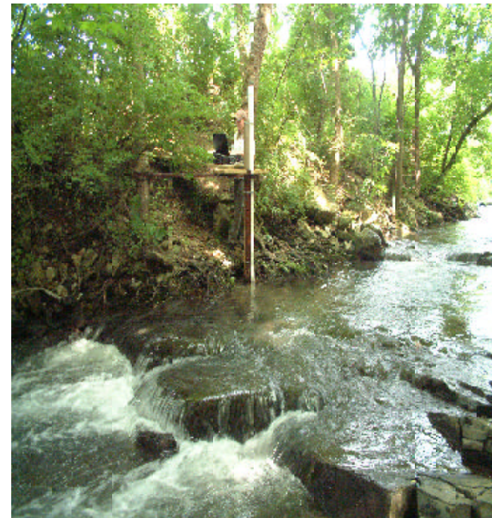
WRMP Technician downloading stream stage data at Thompson Run. Photo by: Todd Giddings
