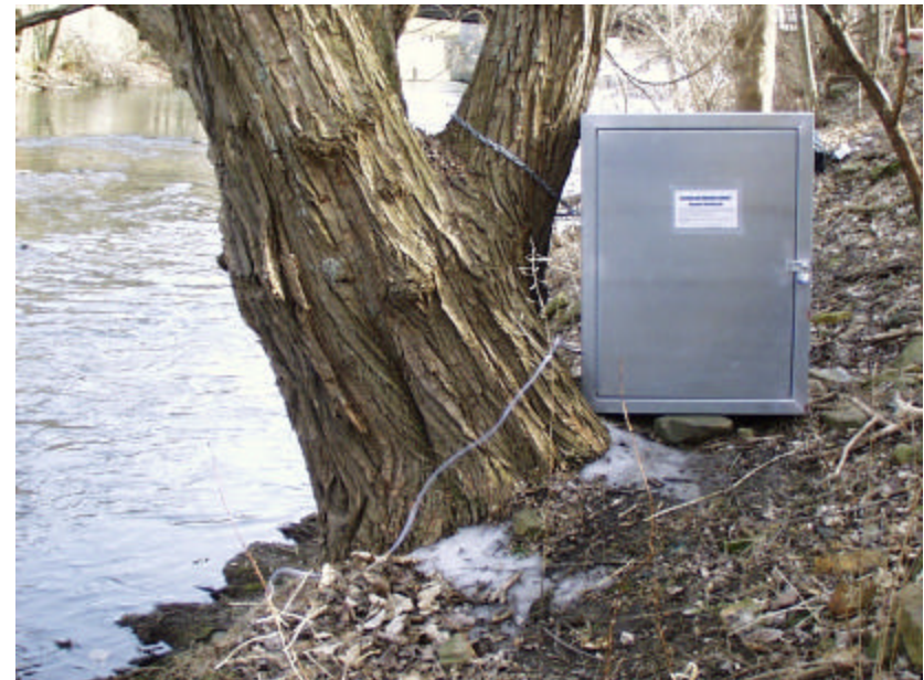
Figure 4. Stormwater sampler at Spring Creek Milesburg.
